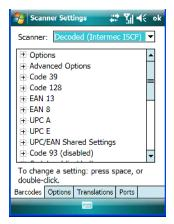
Tap on the Scanner dropdown menu, and choose Decoded (Intermec ISCP).
